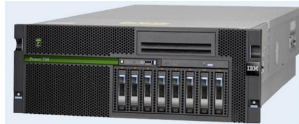
Figure 1. IBM POWER 750 server.
