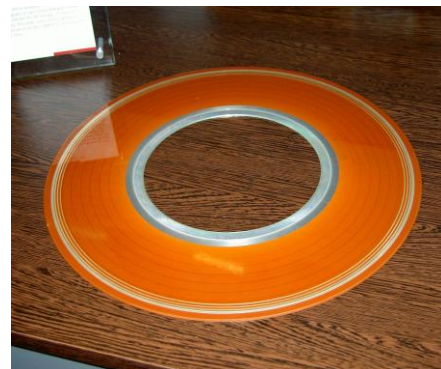
Figure 11. One storage disk showing head crash damage.
